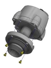
**Note:** This adaptor can also be used with the waveguide option but will require a 36mm pipe. The waveguide pipe should be securely attached via the two grub screws provided and hand tightened with an M1.5 Allen key (Note: over-tightening the grub screws can damage the plastic).
