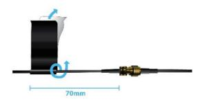
Keep the tape stretched while wrapping, over-lapping half the width of the previous turn.
