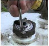
• Place the new gauge of the LPG Logger onto the LPG tank and secure with screws.
