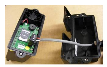
**3.4.** Remove existing battery, replace with new battery ensuring battery connector is wired correctly and inserted into header on the PCB.
